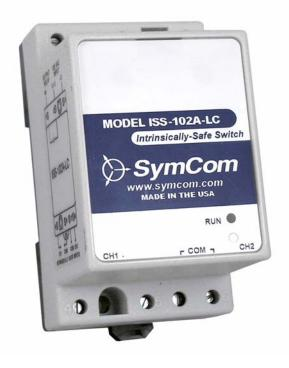
SymCom's ISS-102A-LC (Latching Controller) is a dual-input, single output (form A), pump controller with latching/differential logic. Both input channels are compatible with switches (float, pressure, etc.) and resistive probes (fixed  $100k\Omega$  threshold).
